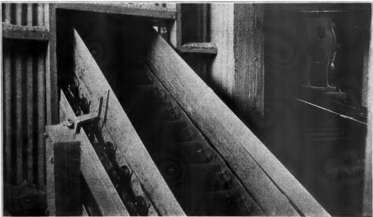
Pan Conveyor From Primary Crusher to Secondary Crusher.
